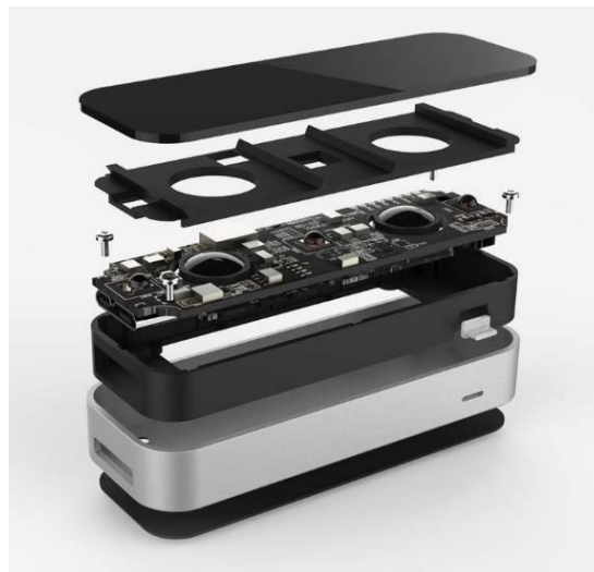
Fig. 3 – Expanded view of the Leap Motion Controller (Leap Motion Developer API Overview, 2015).
